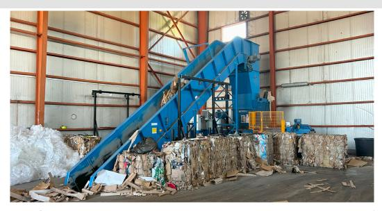
AVE SK specializes in collecting and recycling cardboard and plastic in the area of Bratislava and Senec. A fully automated horizontal baler delivered by FROP, Orwak's distributor in Slovakia, speeds up the operation and helps AVE SK process more recyclables.
