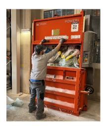
"The balers were very well received by our staff right from the start. The fractions are sorted according to type, and the amount of plastic packaging wrongly discarded as mixed waste is significantly reduced."
