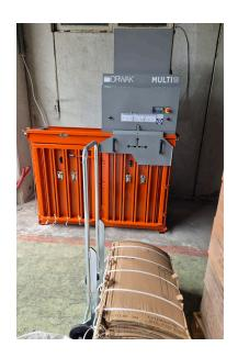
"The multi-chamber vertical baler allows us to simultaneously bale cardboard and plastic foil, the two most important fractions, and in addition to selling them and returning the investment, it results in a more productive use warehouse space."
