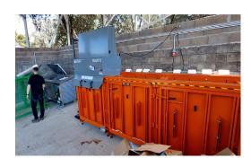
The baler comes with three generous size chambers and works like a mini recycling station for the packaging waste on site. Cardboard, plastic wrapping and aluminum cans are sorted in clean fractions and successfully compacted into dense bales for easy storing, handling and transportation. The bales are delivered to the recycling industry and the new solution is good for the business and the environment.
