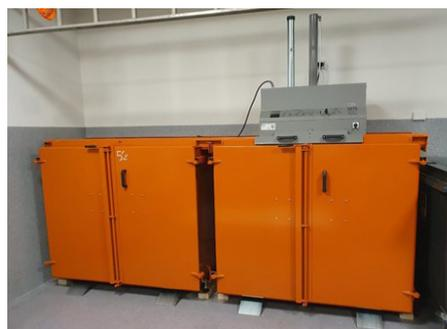
Quality Hotel Ramsalt in Bodø, chose the Orwak multi-chamber baler 5070-Combi, which reduces the amount of residual waste by up to 70 %. This is of great importance for any business focusing on operating costs and on cutting CO<sub>2</sub> emissions. EnviroPac recommended and delivered this multi-chamber solution. The baler is top-loaded meaning that the chambers are open and it is easy to throw waste straight into the two 4-wheel plastic 660 L bins, which are placed in the baler.
