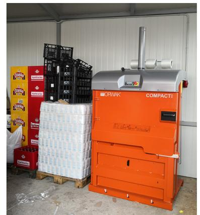
It has a convenient compact design and low height and yet offers a wide loading gate and produces a bale weight in line with what the recycler prefers to pick up. Compact machine design is essential at sites, where the baler will be installed at the second floor and needs to fit into an elevator to get there.
