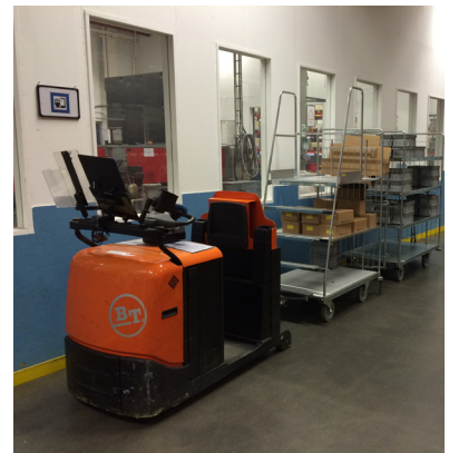
The small electric train supplies components and removes the bales.
