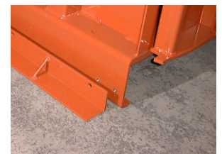
Skid mounting for bolting the machine to the floor
