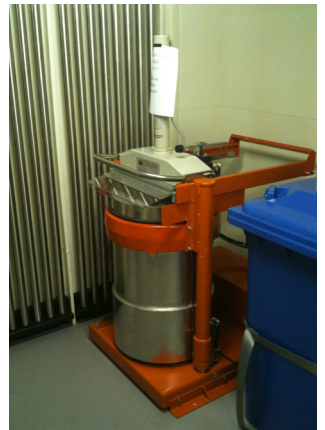
Skid mounting for bolting the machine to the floor
