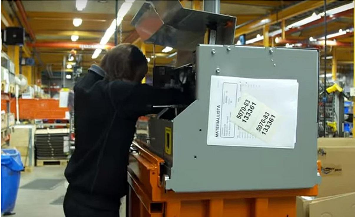
The work is not done just because your new waste management solution is in place and in use. The baler and the briquette press must be cleaned regularly and serviced at least once a year to ensure that they are still functional and safe. It is also important to continuously monitor the operations and the waste streams in your business in order to adapt waste management to possible changes in waste volume and type of material.
